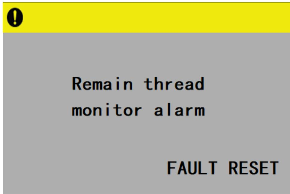
If Bobbin stitch counter reach "0" the machine will stop and alarm, so you can replace the bobbin, then simply click on the fault reset button to continue work.
